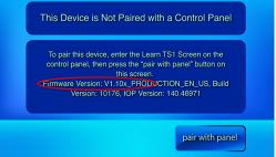
2 Make sure that the Firmware Version on the Control Panel matches the Firmware Version on the TS1 before attempting to "learn-in" or pair the TS1 with the Control Panel.
