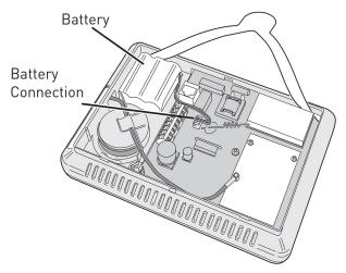
4 Disconnect the power supply from TB1 and 2 on the Control Panel terminal block or unplug the panel power supply from the wall outlet.
