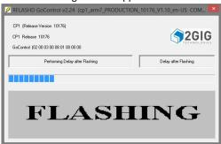
**IMPORTANT:** DO NOT disconnect the cable, the power to the Control Panel, or close the Firmware Update Tool until the status bar has completed and the final screen appears (showing the updated firmware version).
