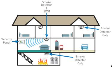
Only one Smoke Detector Sensor is required in an interconnected smoke detection system.
